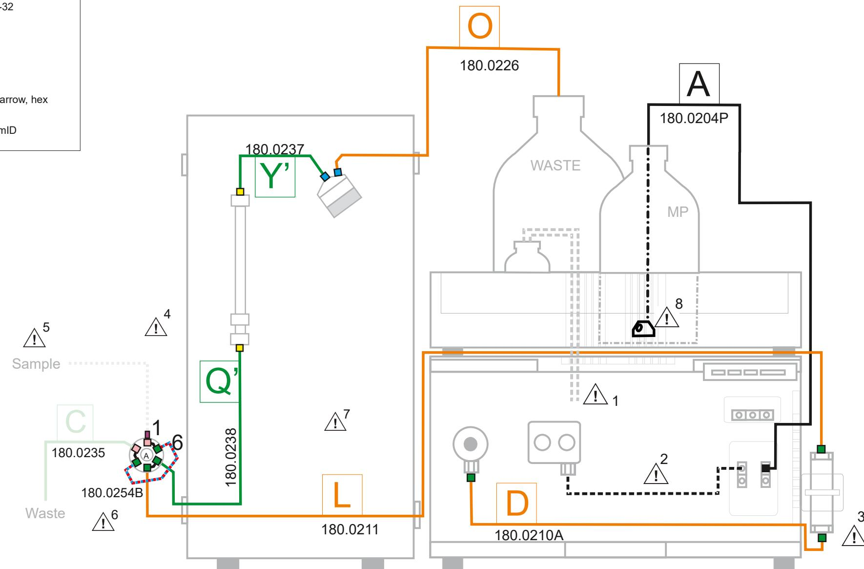
Installation schematics for ALEXYS OMD High Throughput, using
